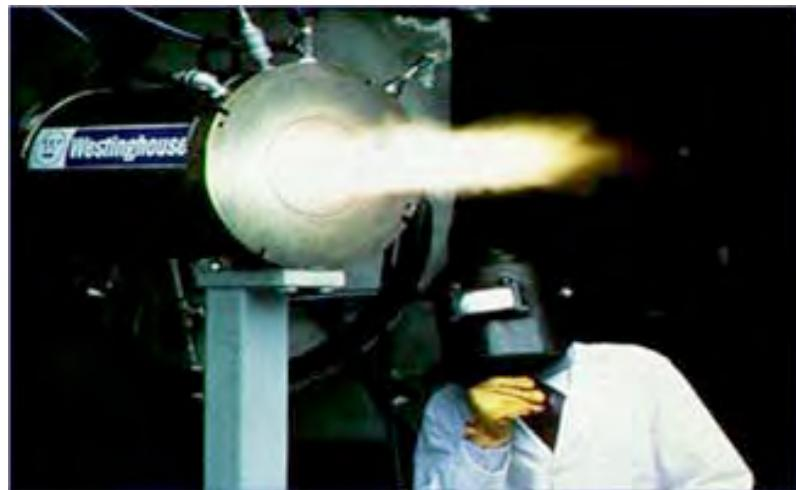
**Figure A-9: Plasma Torch in Operation**
