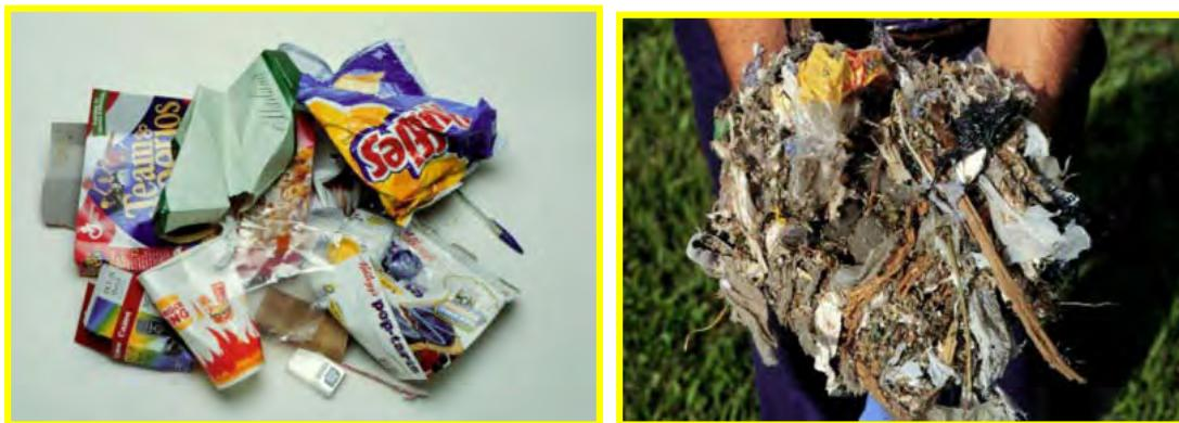
**Figure A-4: Unprocessed MSW (left) and RDF (right) Ready for Combustion**
